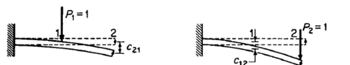
For the same beam, c_{21} = c_{12} . (a) Forces and corresponding displacements.
