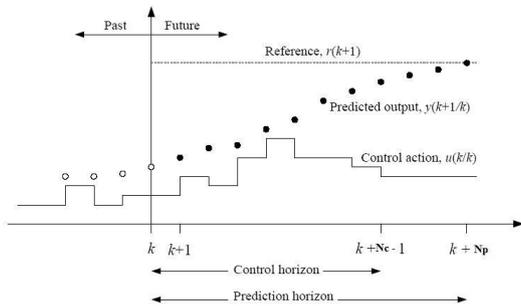
Figure 3. MPC principle
