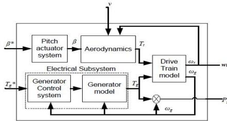
Figure 1. Wind turbine global scheme
