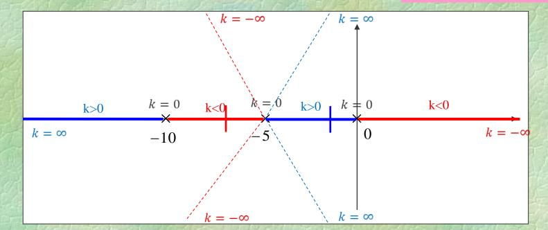
**7- Intersection points of branches with the imaginary axis:** The intersection points with the imaginary axis are found using the Routh-Hurwitz method.
