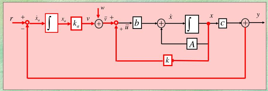
**Exercise 3:** In the above system suppose (A,b) is controllable, and the transfer function  $c(sI-A)^{-1}b$  has no zeros at the origin. Show that the output follows a step in the reference r in steady state
