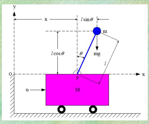
$$M \frac{d^2 x}{dt^2} + m \frac{d^2 x_g}{dt^2} = u - c \frac{dx}{dt} \qquad x_g = x + l \sin \theta$$
