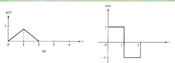
Exercise 6: Find the transfer function and impulse response of the system below.  $\ddot{y} + 2\dot{y} - 3y = \dot{u} - u$
